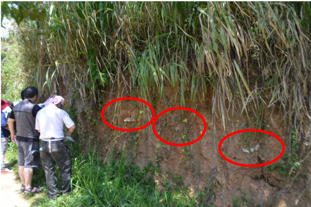
Figure 5: Some debris and plastic waste found in the soil near toe of slope.
